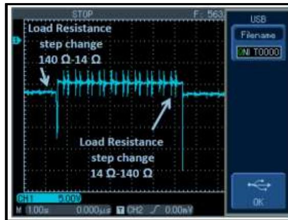
Fig.8 Open –Loop Operation, Buck Mode-Duty ratio = 33%, Input Voltage =24 volt. Output voltage profile for load resistance step changes.
